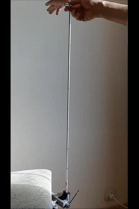
The basic qualitative explanation of the washer's behavior is obvious – it rolls around the rod and due to the centripetal force there is a normal reaction and hence a friction force countering the gravity. As long as the angular velocity is big enough to assure that static friction is bigger than the weight, the washer shall keep its height constant.
